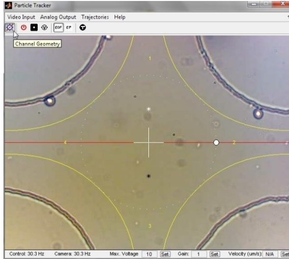
Fig. 7 Graphical user interface (GUI) and coordinate calibration. This simple GUI allows users to select objects, drag them by mouse, draw trajectories for objects to follow, and record experiments. To properly transform between the coordinates used for image processing and those used for control calculations, a schematic of the control device must be dragged, rotated, and scaled to match the image.
